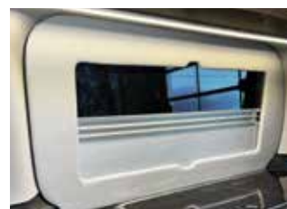
Assembly example: The image shows the undercover window's inner frame behind an interior panel. The panel is not included.
